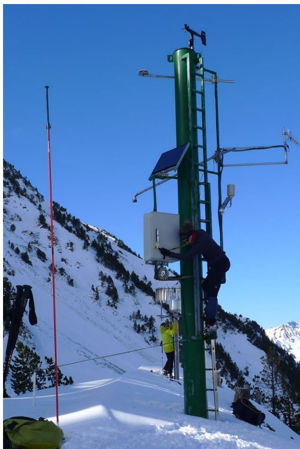
Fig.3.: Dr Laura Trapero looking for the reason of missing snow depth data at the Sorteny meteorological station
