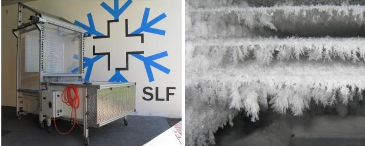
Figure 10. : SnowMaker (left) and nature-identical dendritic snow on the cultivating threads (right).
