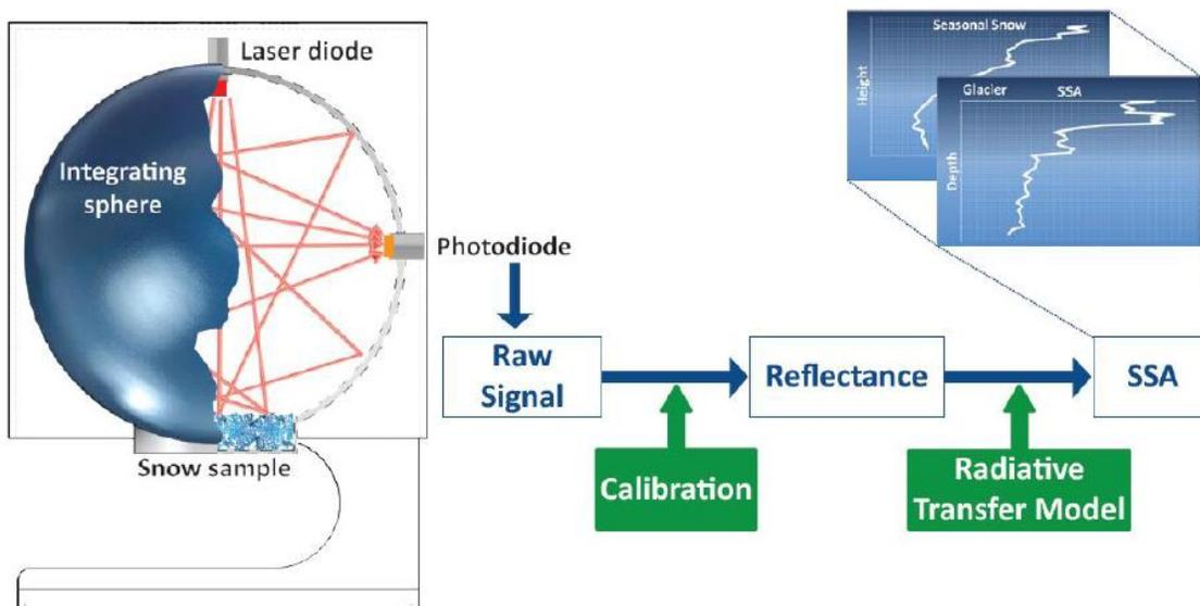
Figure 6. Working principle of laser reflectometer
