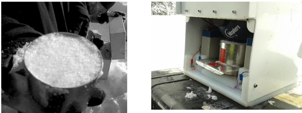
Figure 8. Extracted sample for IRIS measurement (left) Sample is placed inside IRIS under the sphere
