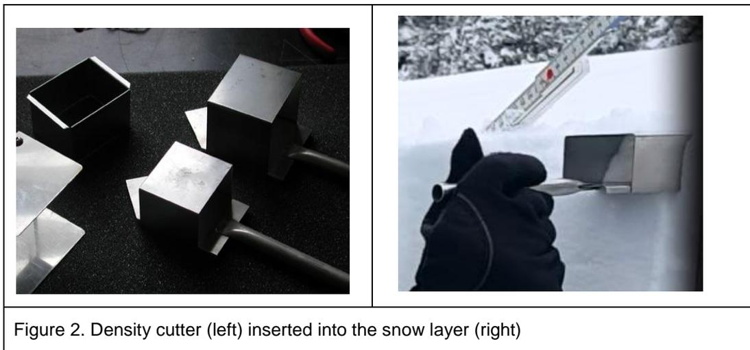
Figure 2. Density cutter (left) inserted into the snow layer (right)
