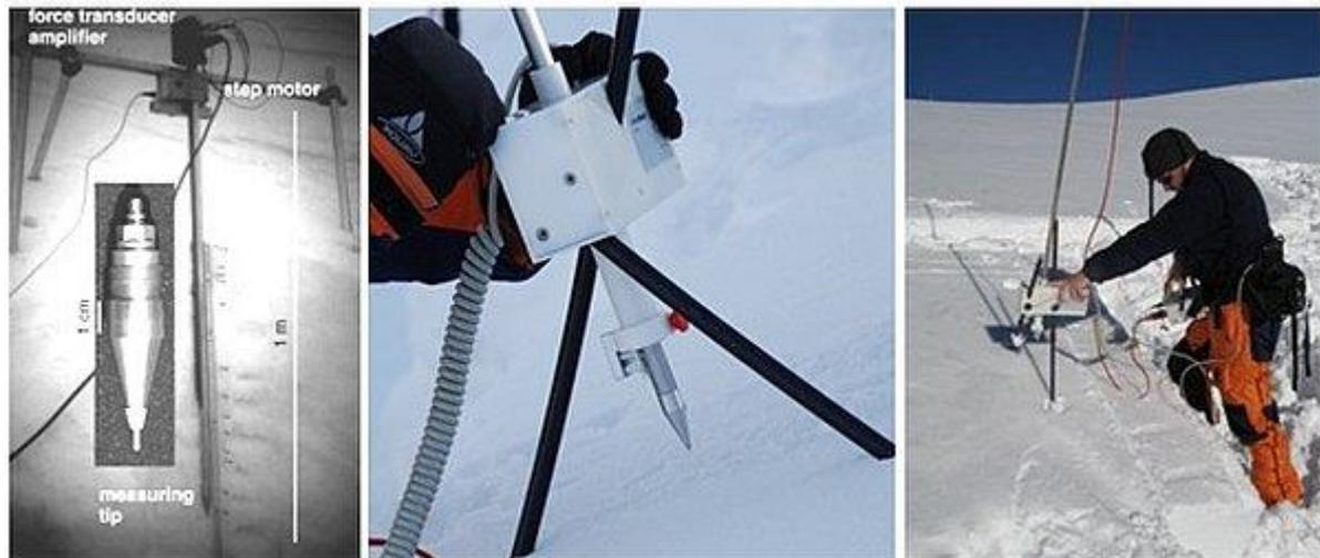
Figure 9. Measuring tip at the end of the rod (left) Motor unit, black poles and the tip (middle) measurement by an SMP (right)
