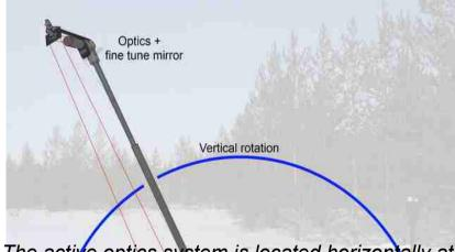
The active optics system is located horizontally at the top of the measuring arm, and is looking down to the target through a mirror. FIGIFIGO consists of the following main components: casing, measurement arm, rugged computer, and a sunphotometer on a tripod.
